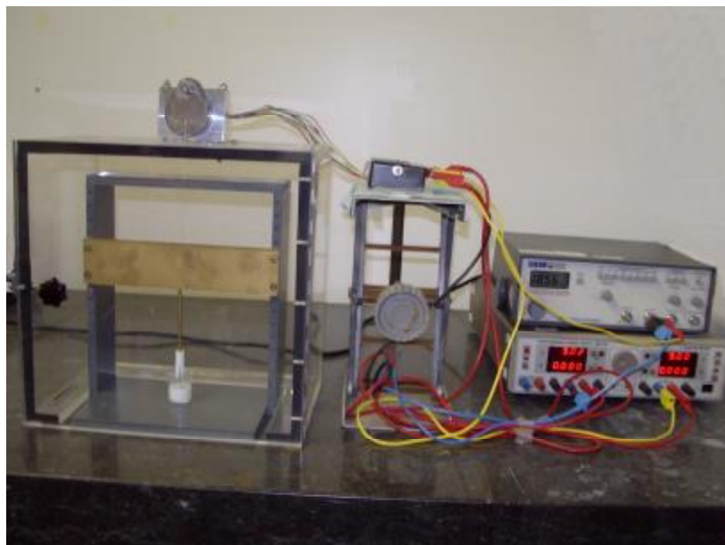
Figure 1. Picture of the home made vertical deposition set-up. The withdrawing
